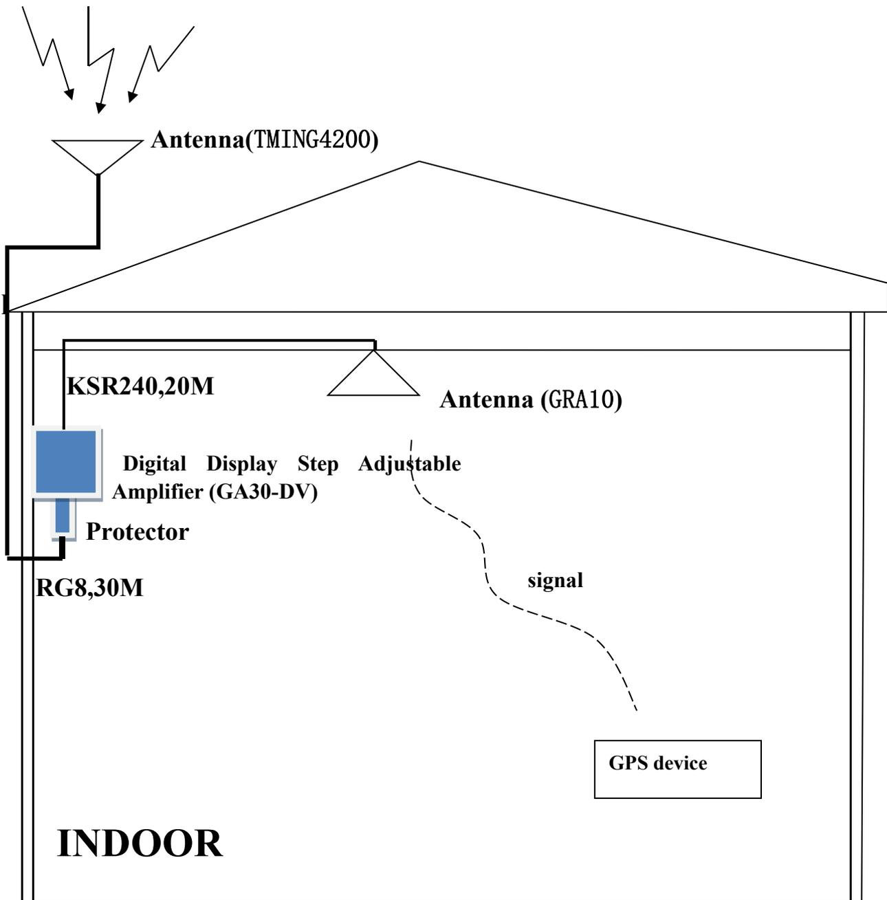
1. GPS/GLONASS/Beidou2/Galileo Antenna(TMING4200) be installed on roof of the building;
