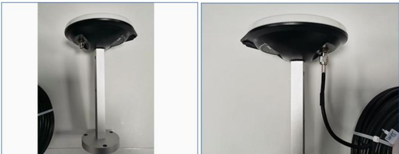
① The feeder joints need to be wound with waterproof self-adhesive tape, starting with the lower part of the joint connection and filling the low-lying part with the tape.
